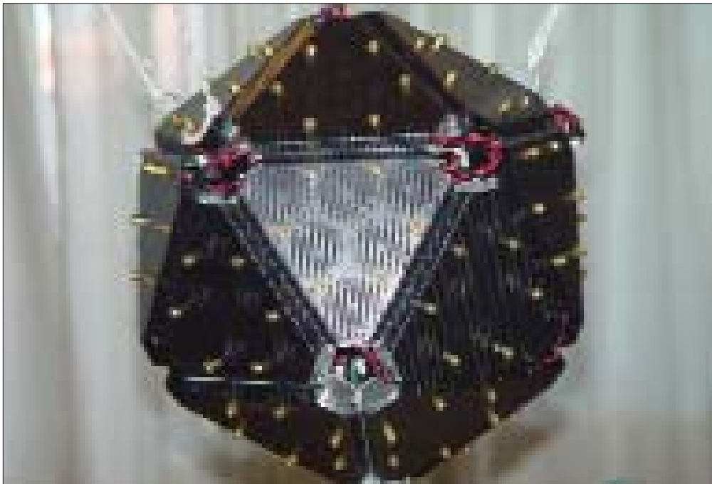
The University of California Berkeley's Center for New Music and Audio Technologies (CNMAT) and Meyer Sound Laboratories have developed a prototype spherical loudspeaker array. It can be used to synthesize radiation patterns of musical instruments, create a monopole source for room measurements, and create directional beams and nulls.
