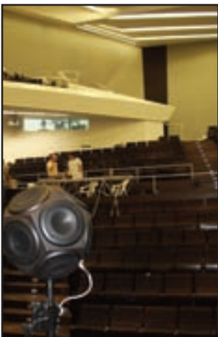
During the tuning procedure, a Dodek is used as an ideal omnidirectional sound source.
