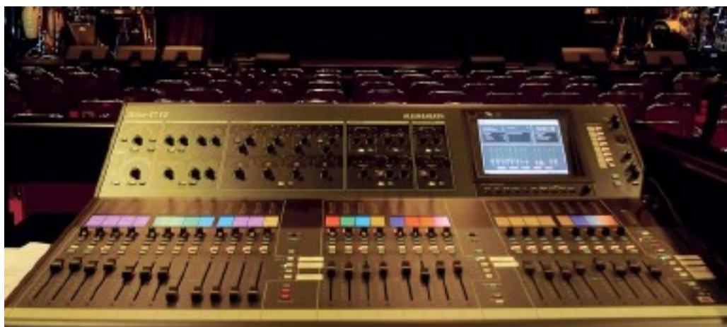
An Allen & Heath iLive T-112 digital console is connected to an iDR-64 Mix Rack at the stage left position
